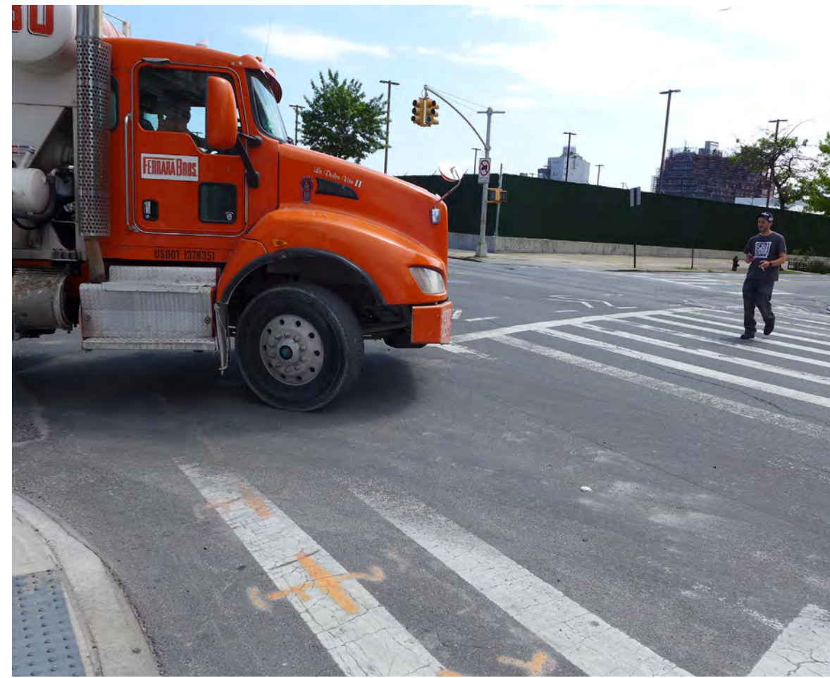
Trucks require large turning radii and wide roadways
